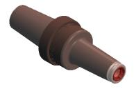
Richards 15kV Loadbreak Elbow Tap Plug (P615ETP)converts a 15/25kV 600A Deadbreak interface (IEE 386 Fig 11) to a 15kV 200 A Loadbreak interface (IEEE 386 Fig 5) for use with a Loadbreak elbow or cap.
